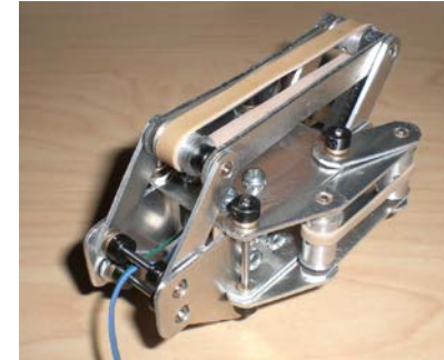
Mobile intestinal imaging robot
