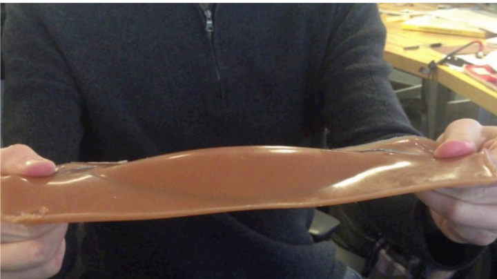
Anisotropic deflection in curved fiber composites
