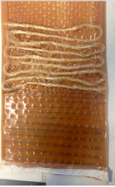
Variable bending stiffness in multi-material woven composites
