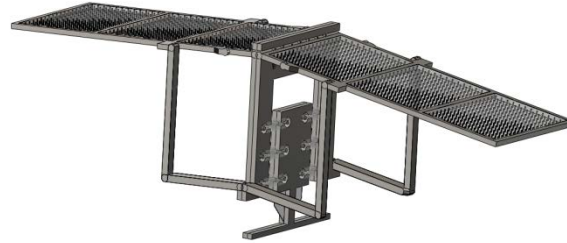
“Pop up” jumping and gliding microrobot
