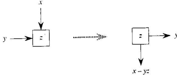
Figure 1-50 The basic operation of a nondiagonal cell in Gaussian elimination.
