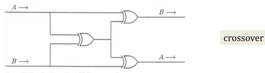
Figure 11. Crossing two wires with three XOR gates.
