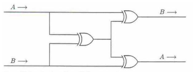
Figure 11. Crossing two wires with three xon gates.
