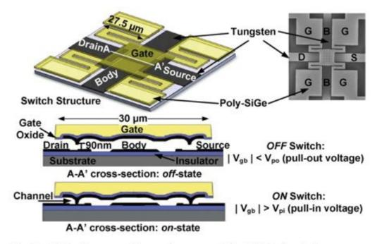
Fig. 1. SEM, diagram, and operating states of the MEM relay device.
