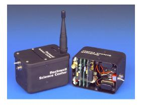
Figure 1: WINS Sensor Node from RSC
