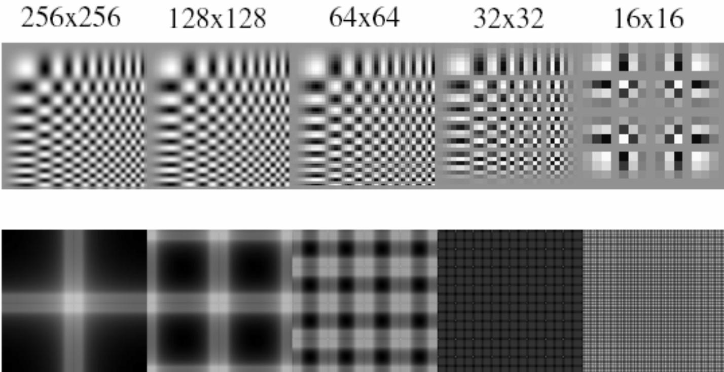
Sampling with smoothing. Top row shows the images. We get the next image by smoothing the image with a Gaussian with sigma 1 pixel, then sampling at every second pixel to get the next; bottom row shows the magnitude spectrum of these images.
