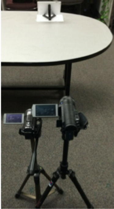
Figure 1. VISIBLE attack setup. Two video cameras are taking a video of the backside of the table as a user inputs keystrokes. Picture taken from [SJC + 16a]
