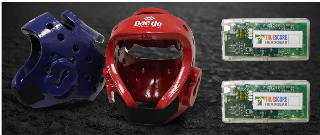
Figure 3: The electronic helmet (e-helmet).
