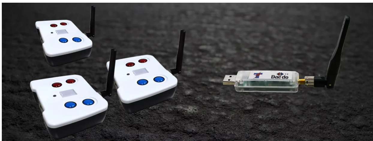
Figure 5: The wireless joysticks and wireless receiver USB dongle.
