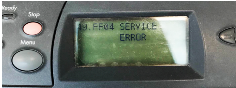
Figure 8: The printer shuts down suddenly after the the buffer overflow attack and display service error.
