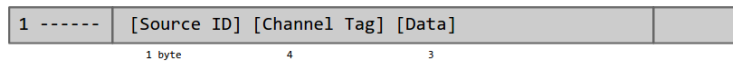
Figure 6: Diagram outlining the general message frame structure for messages devoted to transmitting data on a channel.
