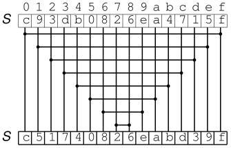
The elements of S are considered as N/2 pairs; each is sorted into increasing order. The input is at the top; the output at the bottom. Horizontal lines represent two-element sorting operations. Crush provides "forward security" for Shuffle.
