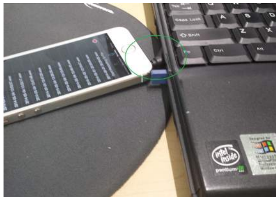
Figure 5: Our final setup is as shown. The green circle indicates where the Dayton Microphone was inserted (in the PCMCIA card slot, which was useful because there were a couple of capacitors close to it).
