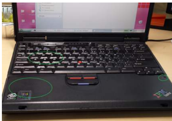
Figure 1: This is the Lenovo Thinkpad T20. The circled regions are where we placed our microphone in order to find the best position to record acoustic leakage. All of these provide a good signal, but we found a better place to put our microphone later.
