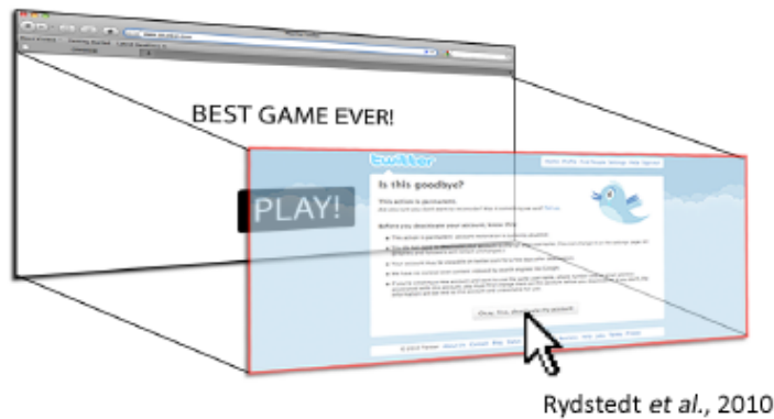
Figure 1 Visualization of a clickjacking attack modeled as a game on Twitter’s account deletion page (Rydstedt et al. 5 ).
