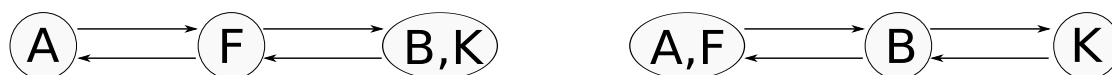
Figure 5: The view of the simplest standalone circuit from the perspective of F on the left, and from the perspective of B on the right.
