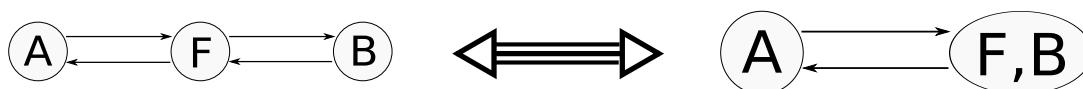
Figure 4: A circuit C containing peers A, B and forwarder F on the left, and how A views this circuit from a tit-for-tat perspective on the right.
