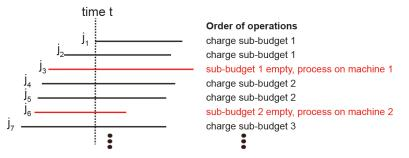
Once we have finished assigning jobs to machines, we "start the clock" on processing. All jobs that are not assigned to machines have this time interval charged to some sub-budget, i.e. some sub-budget gets depleted as processing time passes for the assigned jobs. Once the sub-budget of some job becomes 0 or there is an event such as a job release or a deadline at time t', then we "stop the clock" and repeat the assignment process for  $X_{t'}$ .
