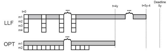
Since LLF still has to process its large job in time [4y, 5y] while the optimal schedule is free, at time 4y, we present both algorithms with a scaled-down version of this same job set (i.e. with y' = y/5) that falls in the interval [4y, 5y]. Again, the optimal algorithm will finish before LLF does. We recursively add scaled-down job sets in this manner until LLF is overloaded and cannot complete the all of the large jobs in each scaled copy before the deadline 5y.
