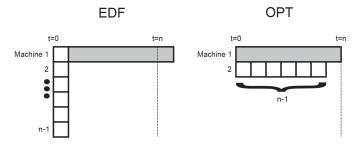
Intuitively, EDF performs poorly on this input because it fails to discern that the large can only be delayed by a short amount of time. On the other hand, each of the small jobs can be can be delayed for quite a long time. We formalize this useful concept below.
