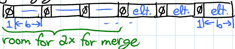
① merge pair of sorted words with  $k \leq \lg n \lg \lg n$  elts. into one sorted word with  $2k$  elts. in  $O(\lg k)$  time
