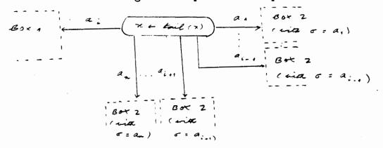
Here Box 2 is replicated for each arrow out of the  $x \leftarrow \text{tail}(x)$  instruction which is labelled with a symbol different from  $a_i$ , and in the replication corresponding to the arrow labelled  $a_j$ ,  $\sigma$  is replaced by  $a_j$ . So
