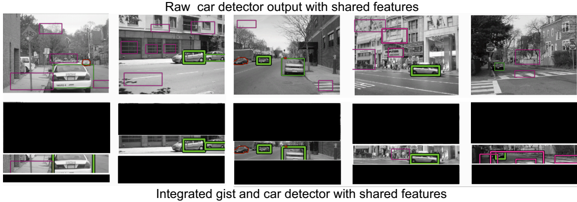
Figure 3.5: Comparison of results obtained when a view-invariant car detector is evaluated on several images (top row), and the results obtained with the integrated hierarchical model (bottom row). Green bounding boxes denote correct detection and red bounding boxes denote false alarms.
