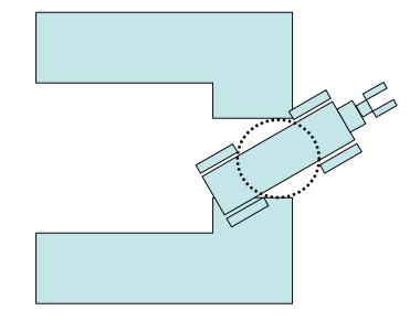
If we make the bounding box the maximum robot dimension, the robot can't find some valid paths
