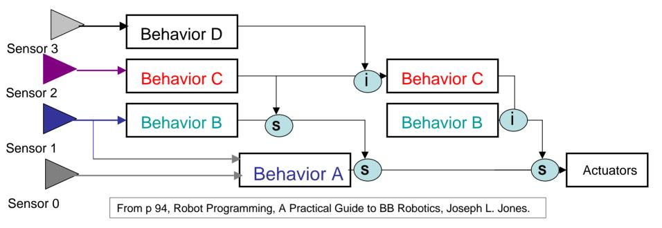
Suppressor node: eliminates lower level control signal and replaces it with one from higher level. Suppression only occurs when higher level is active. Inhibitor node: eliminates lower level control signal without any substitution
