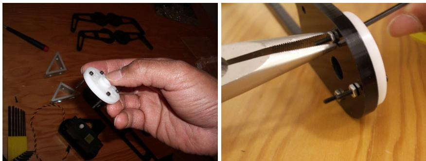
1.1. Mount a large white circular servo horn to C. Use 4 2-56 x  $\frac{3}{4}$ " screw and lock nuts.
