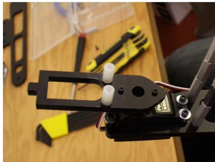
**1.7.** Install the 2 4-40 x 1/2" circular standoffs with 4-40 x 7/16" socket head screws to **G**. On **F**, install an 8-32 x 3/4" metal standoff with an 8-32 x 7/16" socket head screw. Attach the **F** using 2 4-40 x 7/16" socket head screws.
