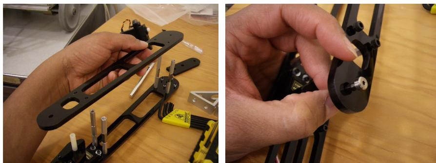
**1.8.** Bolt **D** onto **C** with 8-32 x 7/16" socket head bolts. Use the 3/16" shoulder bolt to fasten **D** to the standoff of **F**.
