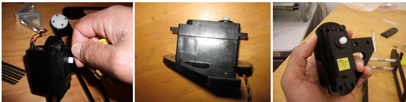
1.3. Install the big servo into I. Make sure you get the servo-flange on the correct side (as seen above). You may have to push hard to pop the servo into place. Use 8-32 x  $\frac{7}{8}$ " screws and lock nuts to secure the servo.
