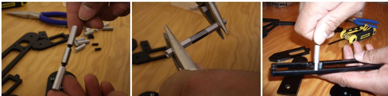
1.2. Screw together three 8-32 standoffs ( $1'' + \frac{3}{4}'' + 1''$ ) to make one 1.75" mega-standoff. Use the 8-32 x  $\frac{1}{2}$ " set-screws. Lock them together tightly with pliers. Make 4 of these and install on C using 4 8-32 x  $\frac{7}{16}$ " socket head screws so that the white servo horn is on the **opposite side** of C from the standoffs.
