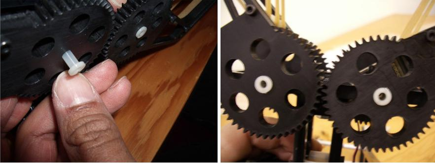
Install each **A** piece onto **J** using a nylon bushing. The bushing should slip through the gripper plate but require some insertion force to push into the wrist-plate. We used the flat side of a closed set of pliers to push with. Secure the bushing with a 2-56 x  $\frac{3}{4}$ " socket head screw and lock nut.
