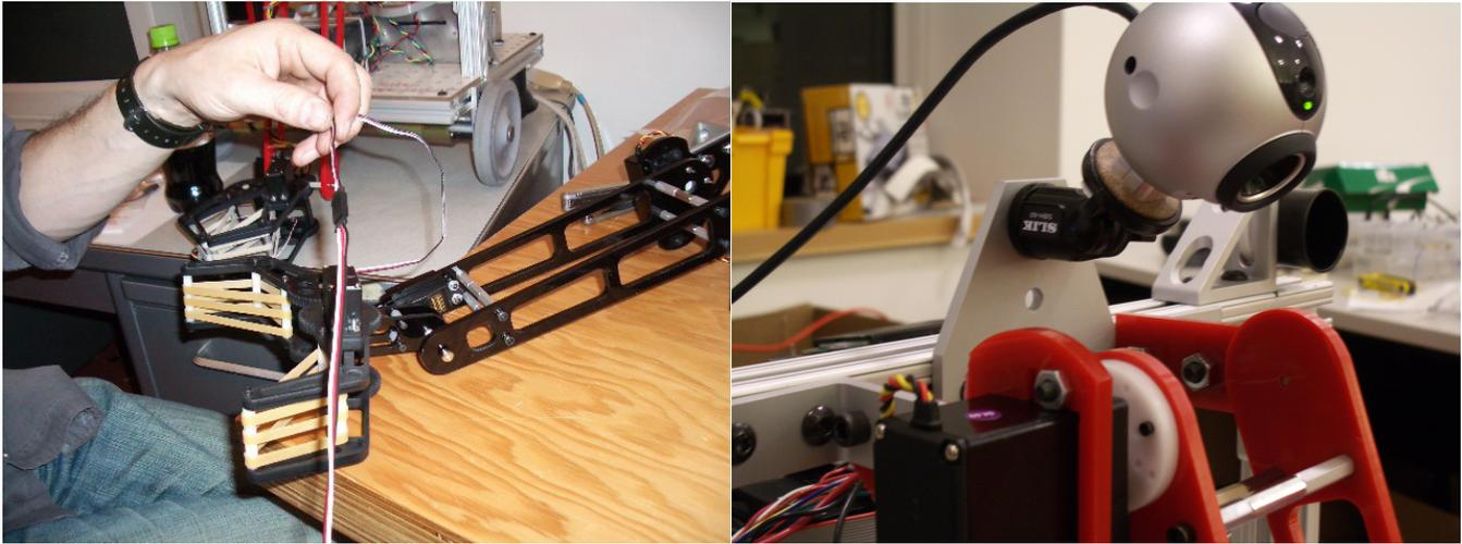
String the wires through the gripper and arm and back to the Orcboard. Use the provided servo extension cables and wire ties to make a clean install. The shoulder must mount to the robot such that the arm clears the camera when it is fully up.
