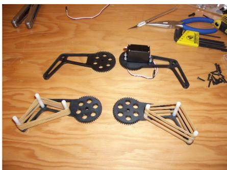
Install the 1.5" standoffs onto the gripper arms **A** and **B** using 6 4-40 x 7/16" bolts. Add three or more rubber bands to each gripper arm.
