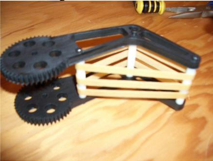
Mount the two gripper-arms together using 6 more 4-40 x  $\frac{7}{16}$ " bolts/
