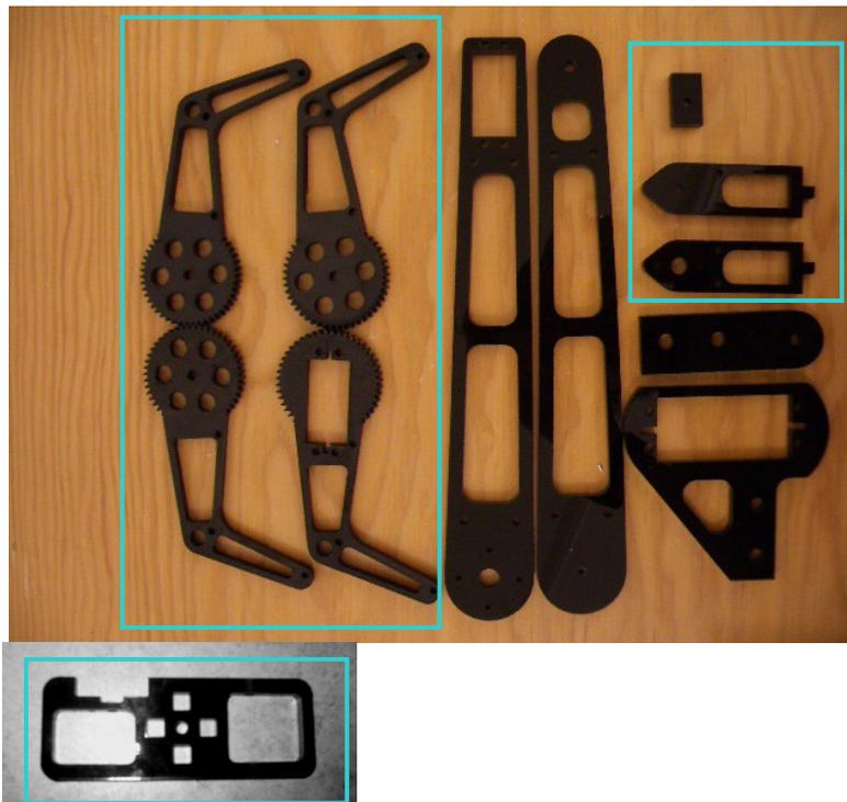
Figure 2: The laser-cut parts for the arm (Wrist mounting plate **J** also needed, but not pictured).
