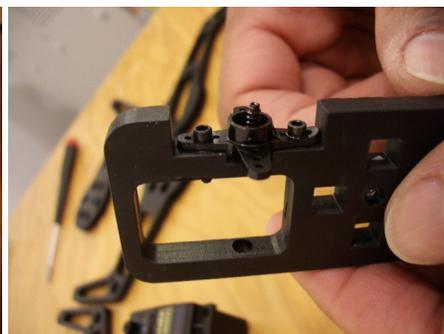
Install the small servo-horn onto the wrist plate, **J**, using short 2-56 socket screws. Note that you must first place the 2-56 x 1/2" servo-horn screw in the horn before mounting the horn to **J**.
