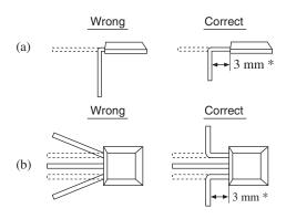
Bending position of lead wire
