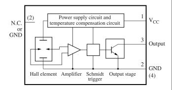
Note) The number in ( ) shows the pin number for the DN6848S.
