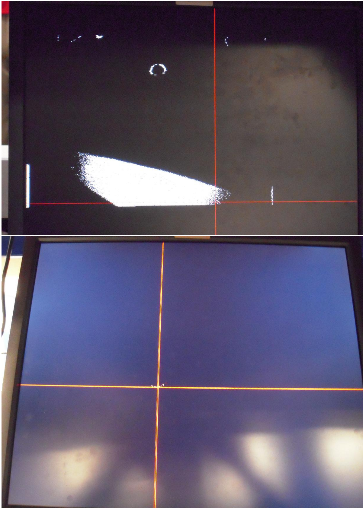
Figure 1: Above: Only red filter applied, noisy video. Below: Red filter and band-pass intensity filter removes extra noise.
