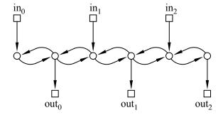
Figure 9.2 A 6-switch packet routing digraph.
