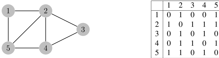
Figure 1: Adjacency matrix representation of an undirected graph.
