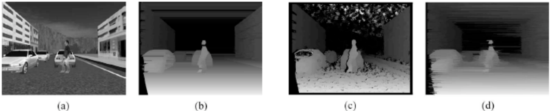
Fig. 6. Results with simulated stereo images. (a) Virtual left stereo image. (b) By S&S DP without noise. (c) By WTA MW5 lr with noise. (d) By S&S DP with noise.
