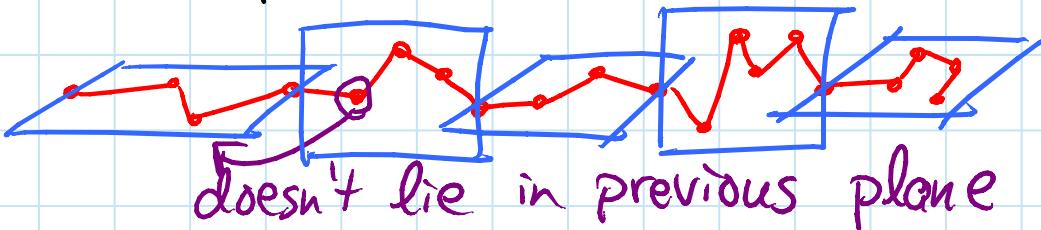
Structure theorem: max span of n-link fixed-angle chain can be partitioned into planar sections each
