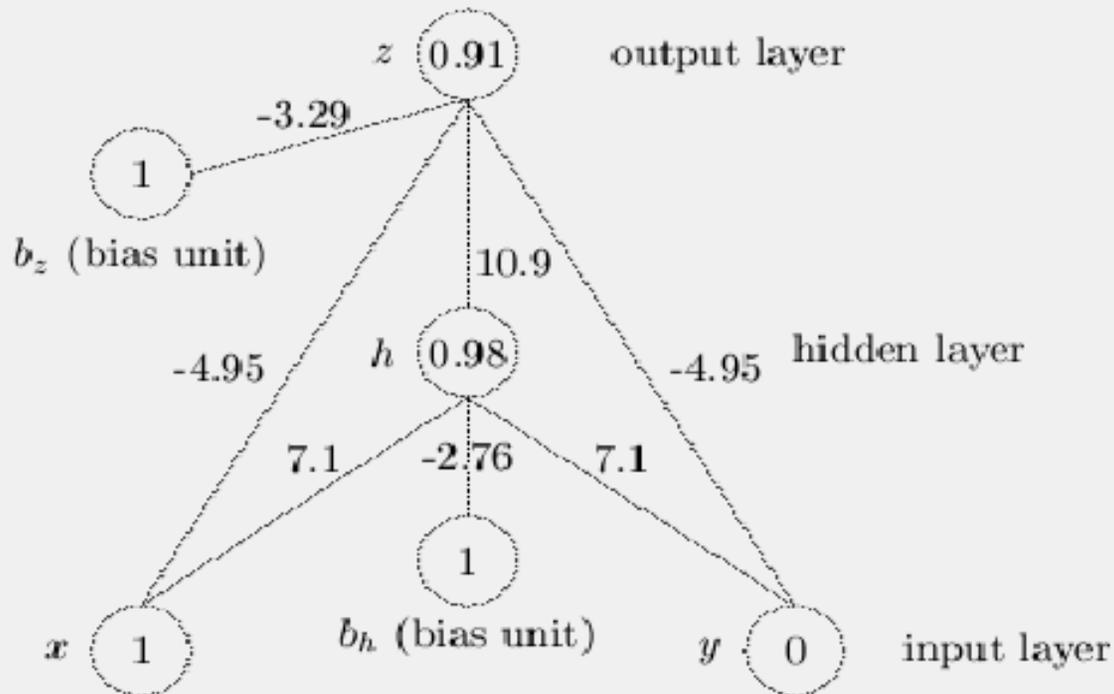
Figure 2.1: A three-layer network to solve the *xor* problem with weights produced by back-propagation.
