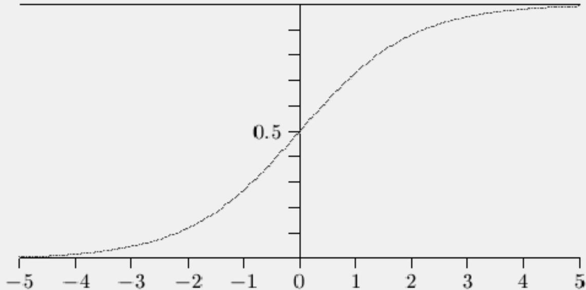
Figure 2.2: A plot of the most commonly used back-propagation activation function,  $1/(1 + e^{-s})$
