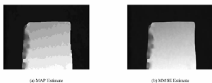
Figure 7. Comparison of MAP and MMSE estimates on a different MRF formulation. The MAP estimate chooses the most likely discrete disparity level for each point, resulting in a depth-map with stair-stepping effects. Using the MMSE estimate assigns sub-pixel disparities, resulting in a smooth depth map.
