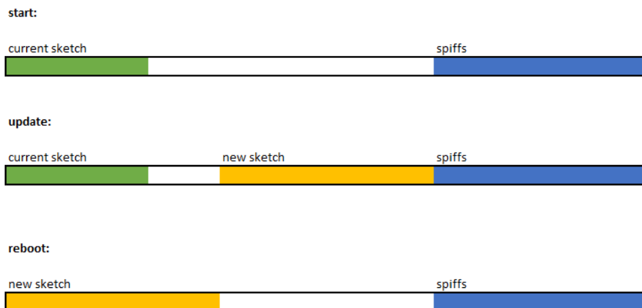
Figure 2: ArduinoOTA writes the new firmware into memory without executing it and checks for signatures before rewriting its current firmware
