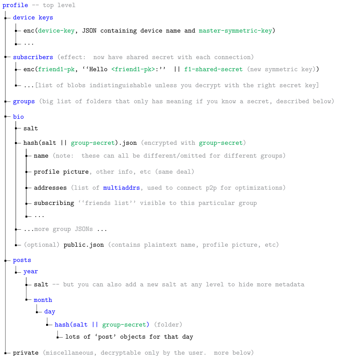
Figure 6: Profile file hierarchy. note: pk = public key (usually friend's RSA key), and all other keys and secrets are symmetric keys
