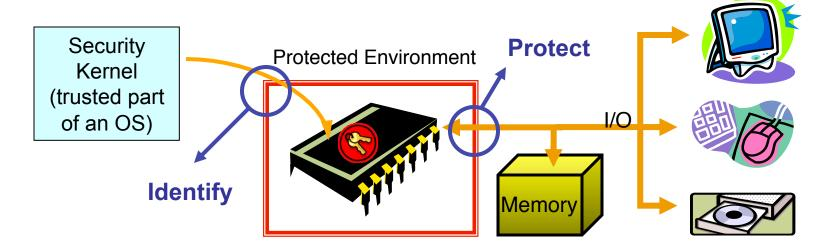
The processor can be authenticated, identifies the security kernel, and protects program state in off-chip memory
