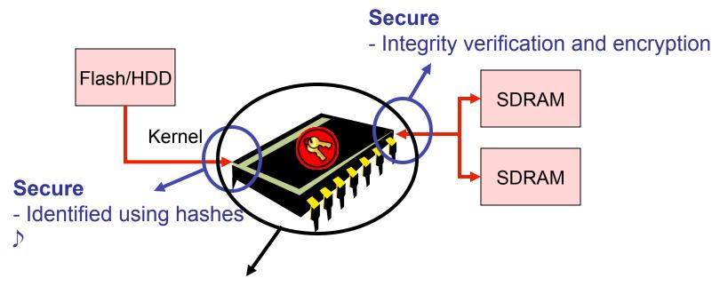
For greater physical security use PUFs and techniques from smart cards and physical intrusion detection circuitry (IBM 4758)
