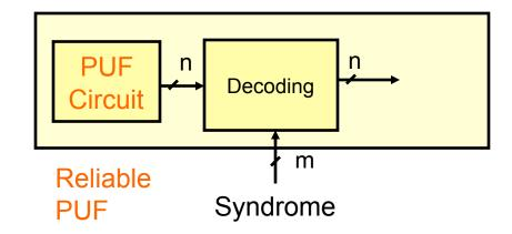
In the field, the syndrome will be used to re-generate the same PUF reference output from the circuit
