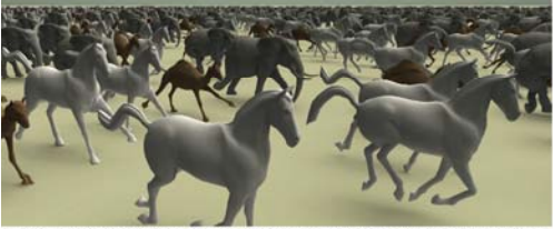
fig 1. Stampede. Ten thousand skinned mesh animations (SMAs) synthesized in graphics hardware at interactive rates. All SMAs are formed using only traditional matrix palette skinning with well-known nonrigid bone transforms. Distant SMAs are simplified.
