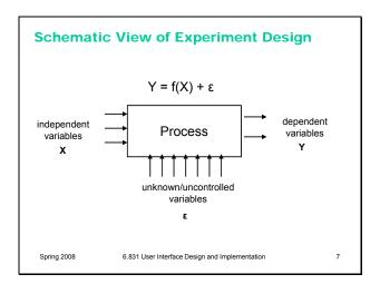
Here's a block diagram to help you visualize what we're trying to do with experiment design. Think of the process you're trying to understand (e.g., menu selection) as a black box, with lots of inputs and a few outputs. A controlled experiment twiddles some of the input knobs on this box (the independent variables) and observes some of the outputs (the dependent variables) to see how they are affected.
