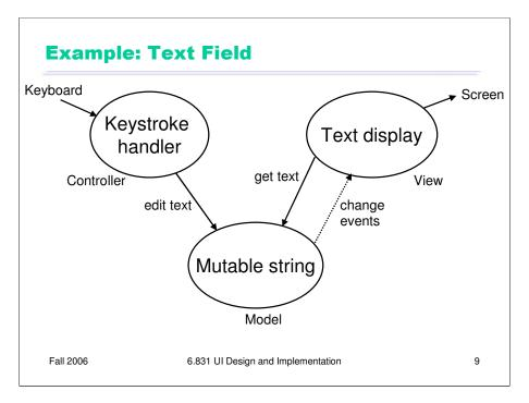
A simple example of the MVC pattern is a text field widget. Its model is a mutable string of characters. The view is an object that draws the text on the screen (usually with a rectangle around it to indicate that it's an editable text field). The controller is an object that receives keystrokes typed by the user and inserts them in the string.
