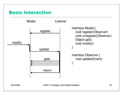
Here's the conventional interaction that occurs in the observer pattern. (We'll use the abstract representation of Model and Observer shown on the right. Real models and observers will have different, more specific names for the methods, and different method signatures. They'll also have multiple versions of each of these methods.)
