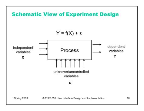
Here's a block diagram to help you visualize what we're trying to do with experiment design. Think of the process you're trying to understand (e.g., menu selection) as a black box, with lots of inputs and a few outputs. A controlled experiment twiddles some of the input knobs on this box (the independent variables) and observes some of the outputs (the dependent variables) to see how they are affected.
