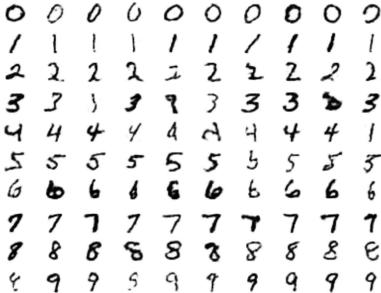
Figure 5: Each row shows 10 samples from the generative model with a particular label clamped on. The top-level associative memory is run for 1000 iterations of alternating Gibbs sampling between samples.
