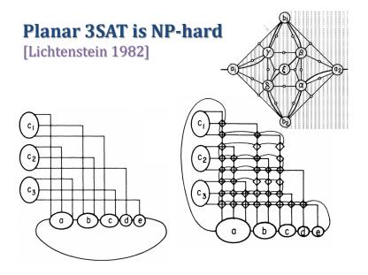
Figure 3: Planar 3SAT with a cycle through variable nodes. Top right: the path through the crossover gadget. Left: the initial arrangement of the bipartite graph, with the variables in a cycle. Bottom right: the arranged graph, with crossover gadgets inserted to preserve planarity; note that some gadgets are required to cross the path across an edge rather than to cross two edges over.
