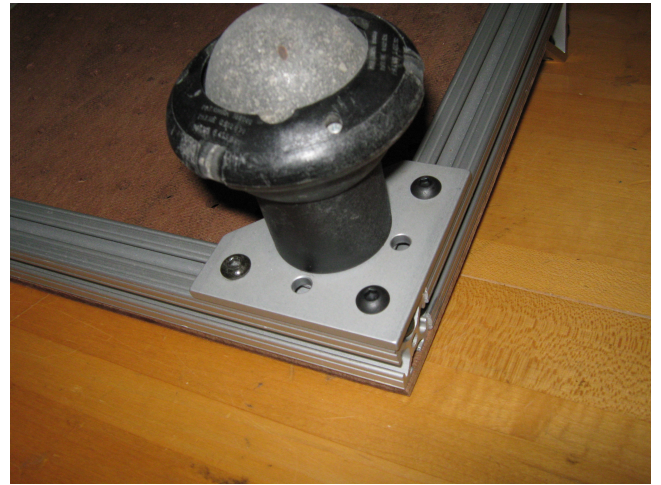
Figure 8: Tighten the casters onto the two rear corners.
