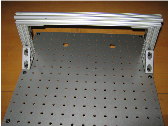
Figure 9: Attach the rollbar to the angle brackets on the top of the robot.
