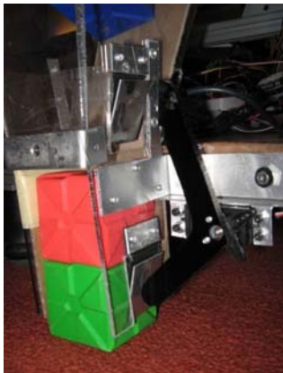
Block marshalling, servo-controlled release mechanism
