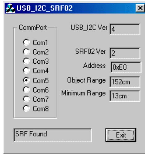
Connecting the SRF02 to your PC via USB is this easy. The USBI2C module supplies the SRF02 with power directly from the USB bus. The USB\_I2C\_SRF02 program can be [downloaded here](#).
