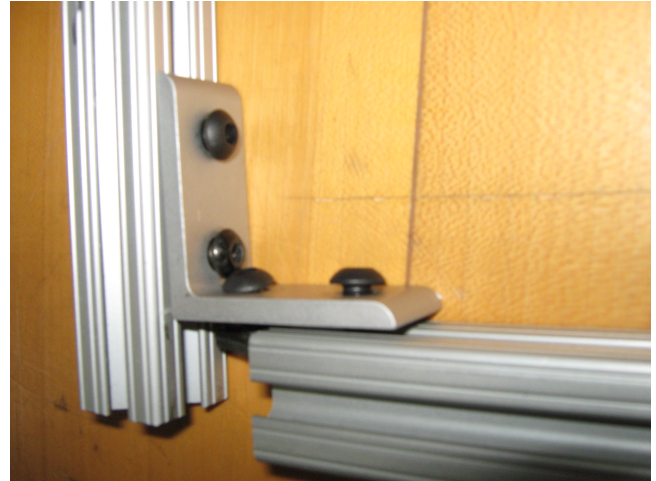
Figure 2: Slide the 5'' segments of 80/20 onto the L-brackets.
