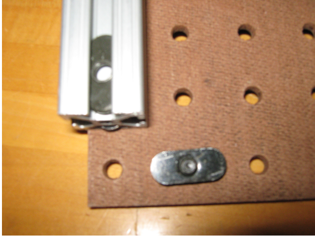
Figure 7: Slide the final piece of 80/20 onto the rear end of the robot.
