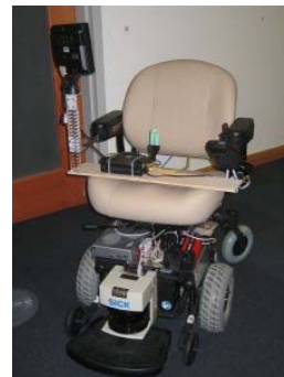
Voice-commandable autonomous wheelchair
