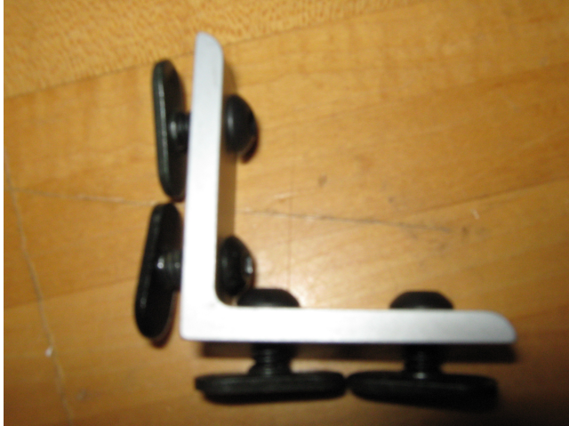
Figure 1: Rollbar assembly: Put bolts and sliders on the L-brackets.
