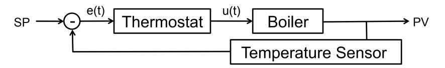
How could the function **u(t)** be implemented? u(t) = **1** if e(t) > 0 [i.e., if SP > PV], **0** otherwise
