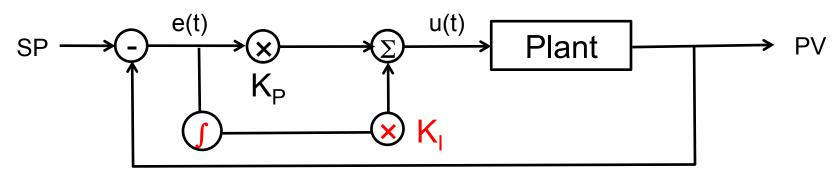
Then  $u(t) = K_P \times e(t) + K_I \times \int e(t)$  (where the integral of the error term is taken over some specified time interval) This produces a *proportional-integral* (PI) controller
