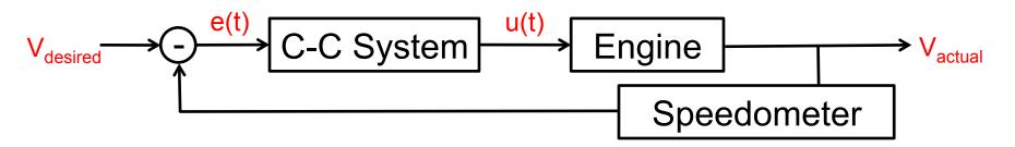
Define  $e(t) = V_{desired} - V_{actual}$ ,  $u(t) = K_P \times e(t)$ , clipped to [0..1] i.e. Throttle =  $K_P \times (V_{desired} - V_{actual})$ Does this controller "settle" at the desired speed? No; it exhibits **error** (E).
