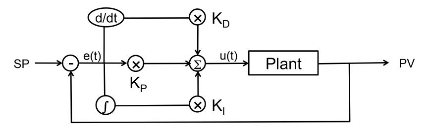
Then  $u(t) = K_P \times e(t) + K_I \times \int e(t) + K_D \times d[e(t)] / dt$ This is a "proportional-integral-derivative" or *PID controller*
