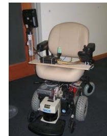
Voice-commandable autonomous wheelchair
