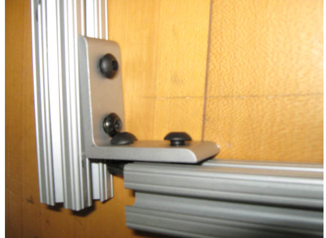
Figure 4: Slide the 5" segments of 80/20 onto the L-brackets.
