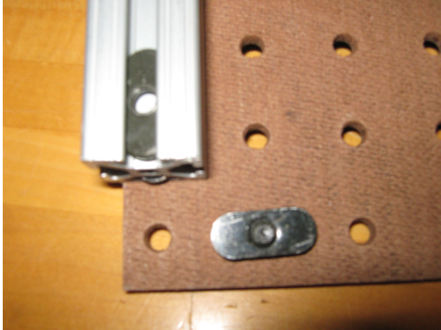
Figure 9: Slide the final piece of 80/20 onto the rear end of the robot.
