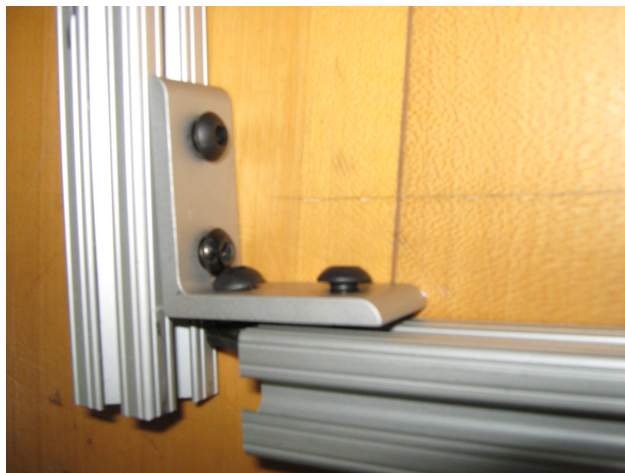
Figure 3: Slide the 5'' 80/20 onto the L-brackets.
