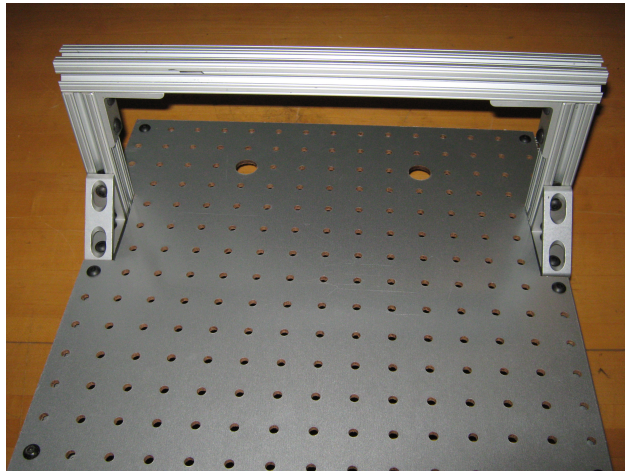
Figure 10: Attach the rollbar to the angle brackets on the top of the robot.
