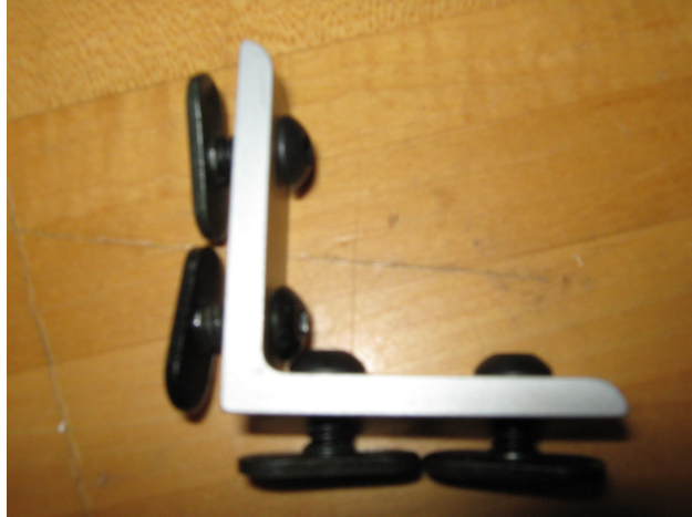
Figure 2: Rollbar assembly: Put bolts and sliders on the L-brackets.
