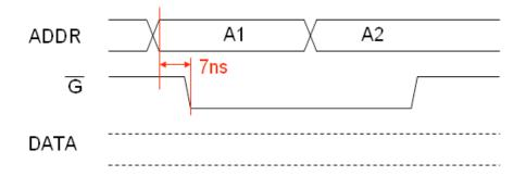
(B) The timing diagram below shows a single WRITE access. Complete the timing diagram, drawing a detailed plot of the DATA signal showing when it must be valid with respect to the write enable (Wbar) control signal. Anotate your diagram with times derived from the data sheet, showing the necessary timing relationships between ADDR, Wbar and DATA. Assume that the chip's enable signals (E1bar, E2) are asserted and that the output enable (Gbar) is deasserted.
