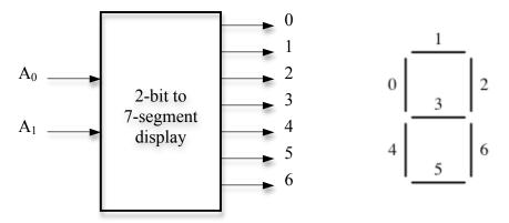
Given the appropriate binary input, this decoder produces outputs that light up the display in the following manner:
